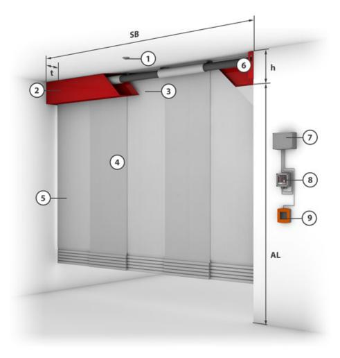
1 = Smoke detector 2 = Casing 3 = Side guide 4 = Fixing bracket 5 = Fabric 6 = Closing element 7 = Tubular motor
