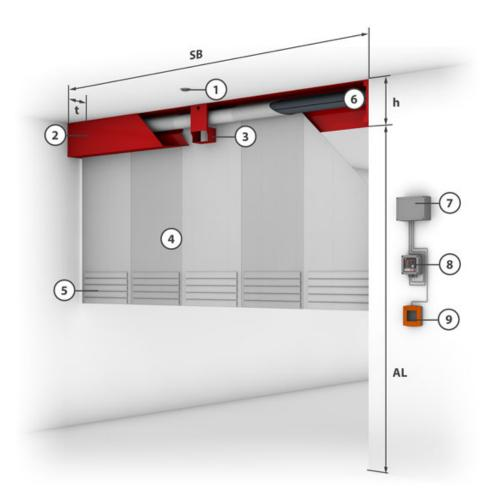
1 = Smoke detector 2 = Casing 3 = Side guide 4 = Fixing bracket 5 = Fabric 6 = Closing element 7 = Tubular motor
