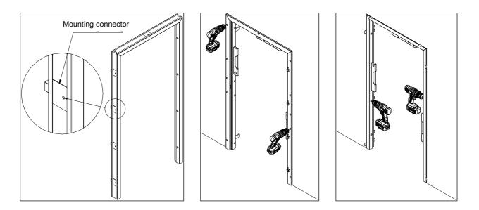
Fasten the frame through the existing mounting holes and underlying mounting connectors in the frame. Drill holes through the mounting holes and fasten the frame with the supplied fasteners. Any counter frame is also fastened through the prepared holes for mounting.
