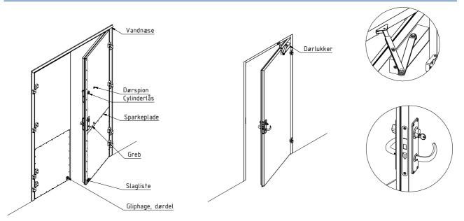
When the frame is mounted in the wall opening and all measurements are checked, the door leaf is mounted on the hinges on the frame.
