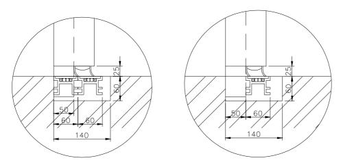
The threshold is delivered either welded on the frame or detached.
