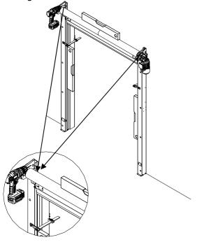
2. Possible lifting gear are removed and the blade are pushed into the sliding rail in the legs. The frame legs are adjusted to the door blade by moving it up and down. The door is moved up/down manually by using the delivered allen key or a power drill with a long allen bit for drill.
