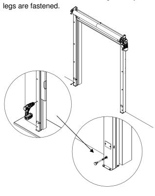
4. The legs are fastened into the floor.
