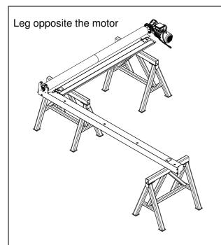
Frame leg is fastend on the internal side of the bearing, as close to the roll as possible.
