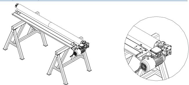
The roll with attached motor is placed in a way that both ends are free for mounting.
