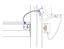
The photocells are brought down in each frame leg and fastened in the prepared connectors.
