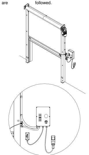
The junction box for the spiral cable is fastened to the frame leg in the prepared holes and the cables are connected to the control box.
