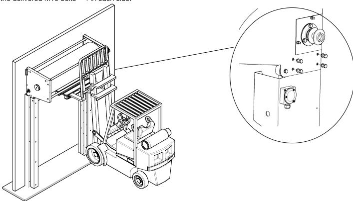
The door is lowered until the framelegs reaches the floor. Make sure the roll is in level and centered above the wall opening, if needed the frame legs are jacked up. The roll is fastened to the wall with the delivered fasteners.
