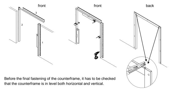
The counter frame is prepared with mounting holes and underlying mounting connectors where the counterframe has to be fastened. Drill holes through the mounting holes and fasten the counterframe with the supplied fasteners.
